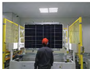
层压后目检 Visual inspection
